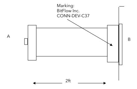
Connector A is a 40 pin mass termination connector with a single center key. The cable at connector A comes out on the opposite side of the polarizing key. There is no strain relief on A.
