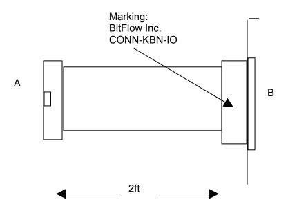
Connector A is a 60 pin mass termination connector with a single center key. The cable at connector A is on the same side like the polarizing key. There is no strain relief on A.
