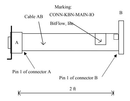
**Connector B** is a 60 pin, two row press fit female connector. Connector B should have **only one center key.** Do not install strain relief. Cable should exit connector on side of the center key.
