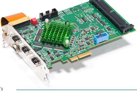
The Axion-CL is BitFlow's 6th generation Camera Link frame grabber. We have used years of experience to engineer the best CL frame grabber in existence.
