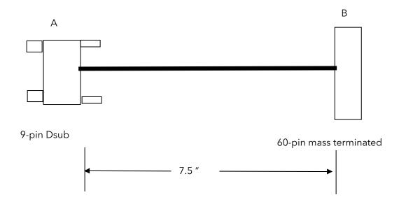
**Connector A** is a 9-pin female Dsub that can be installed on a PC bracket. It has female locking screws to mate with a corresponding male Dsub.
